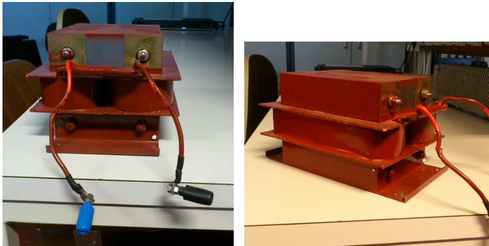
Figure 4.1: Front and side view of short UI transformer.
